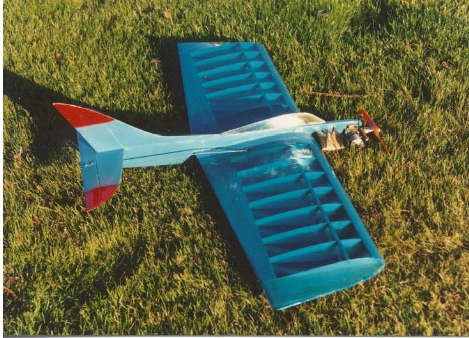
Testor's Flite Streak, Designed by George Aldrich. One of the best flying kits ever! Great airplane for Combat, Stunt or anything else. The CG goes on the SPAR!
